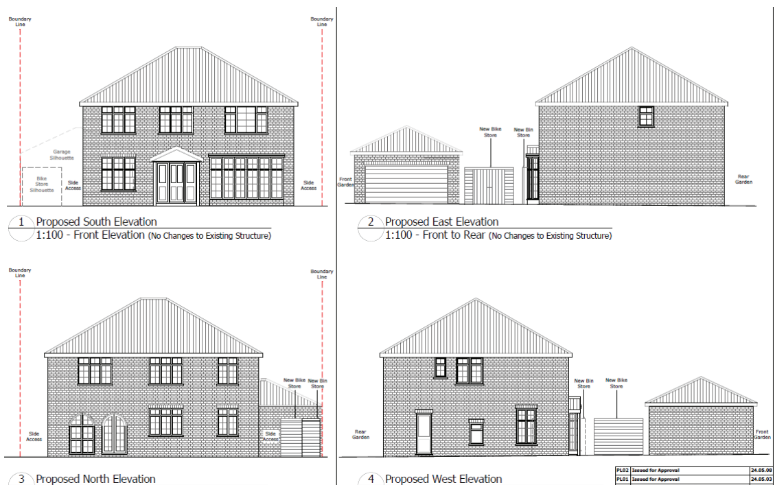
Figure 4: Proposed Elevations (please note – larger version of plan can be found in the Committee Plan Pack)
